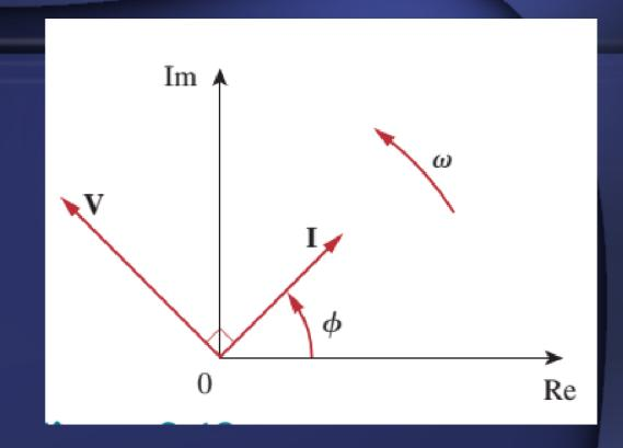
showing that the voltage has a magnitude of  $\omega LI_m$  and a phase of  $\phi + 90^{\circ}$ . The voltage and current are 90° out of phase. Specifically, the current lags the voltage by 90°. Figure 9.11 shows the voltage-current relations for the inductor. Figure 9.12 shows the phasor diagram.
