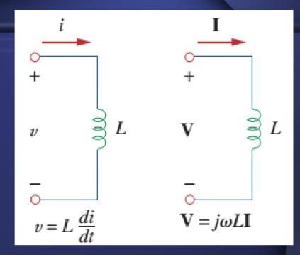
$$\mathbf{V} = \omega L I_m e^{j(\phi + 90^\circ)} = \omega L I_m e^{j\phi} e^{j90^\circ} = \omega L I_m / \phi + 90^\circ$$
